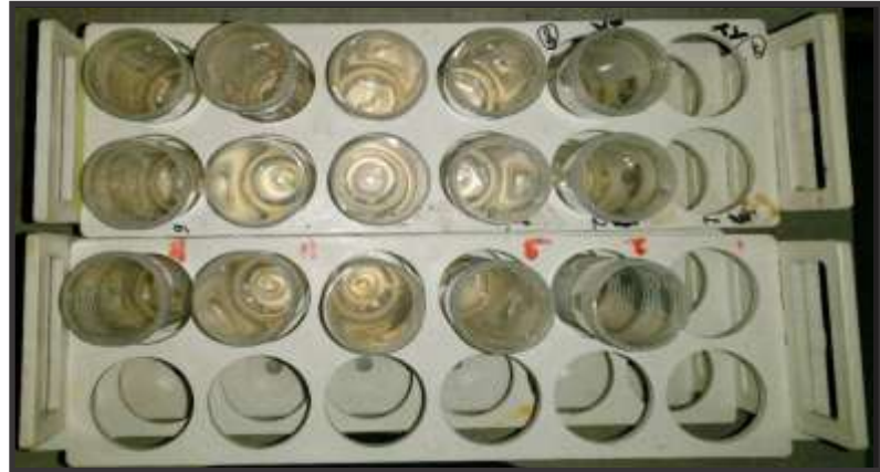
Sample immersion in 10ml of chelating agents for 2 minutes
