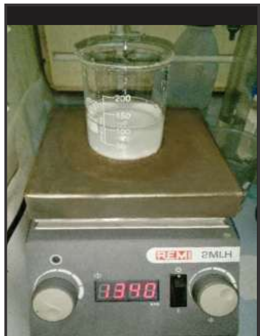
Salt was added in 100ml of distilled water in a magnetic stirrer bath for 1 hour
