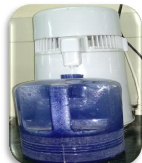
Fig 20: Distilled water plant
