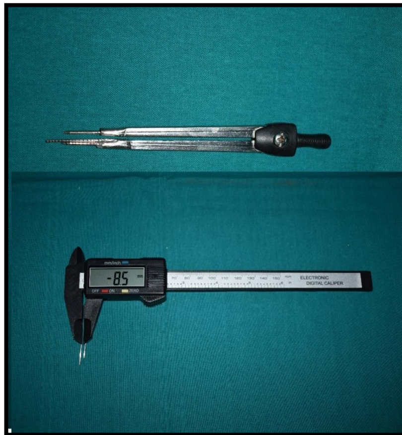
Fig. 4: Modified divider & Modified Digital Calliper shown respectively
