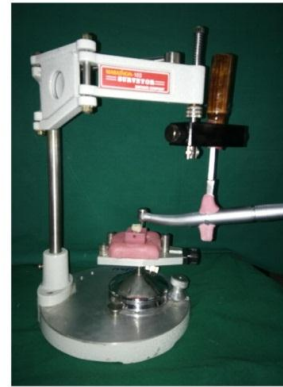
Fig. 29 Mounted assembly on surveyor for tooth preparation
