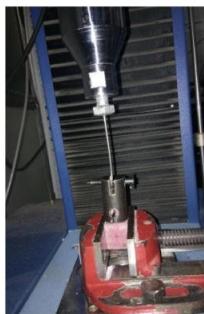
Fig. 50 Retention testing in UTM
