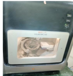
Fig. 41 Milling of copings
