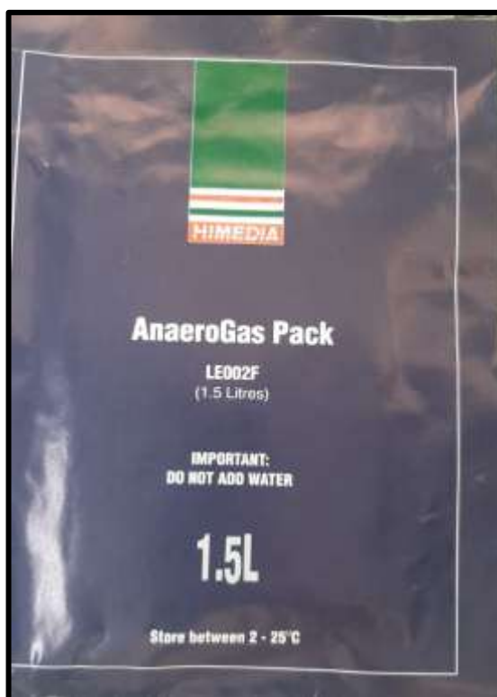
Fig.14- anaerobic pouch for incubation of anaerobic organisms
