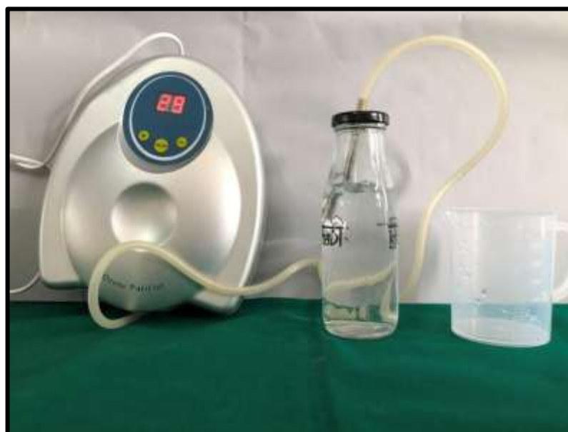
Fig.16- Preparation of ozonated water through bubbling of ozone gas in distilled water
