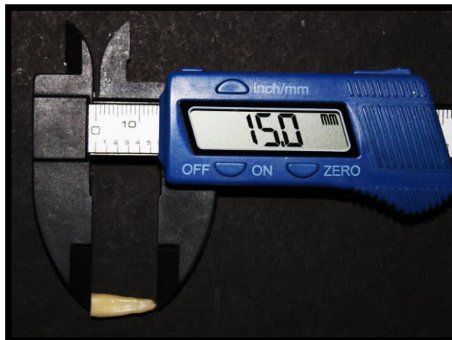
Length Measured with Digital Vernier Caliper
