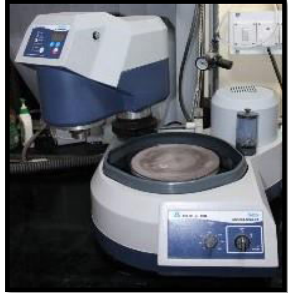
Polishing of samples on Grinder & polisher (Buehler)
