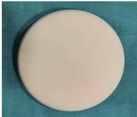
Fig. 1: CAD CAM milled Polyetheretherketone.
