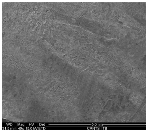
Fig. 28: SEM analysis of CAD CAM sample at bonding failure under 40X
