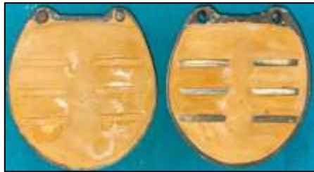
Fig 17: Preparation of gypsum mould
