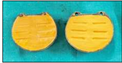
Fig 18: Molds to obtain heat cure PMMA and Bis-Acryl samples
