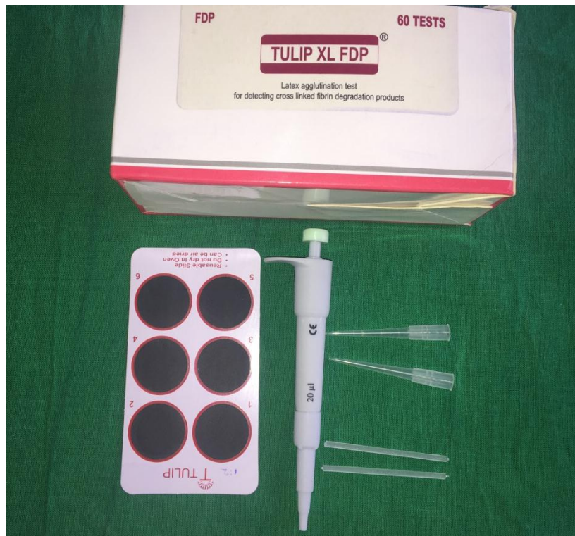
Plastic slide with six reaction circles, disposable sample dispensing dropper, mixing sticks.
