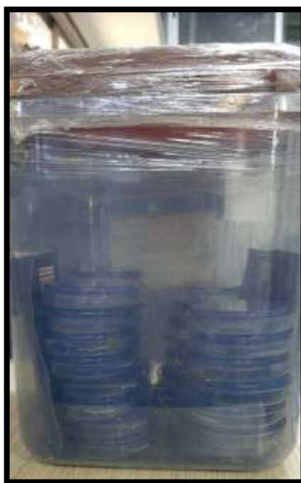
Fig. 22 Anaerobic jar with Gas packs
