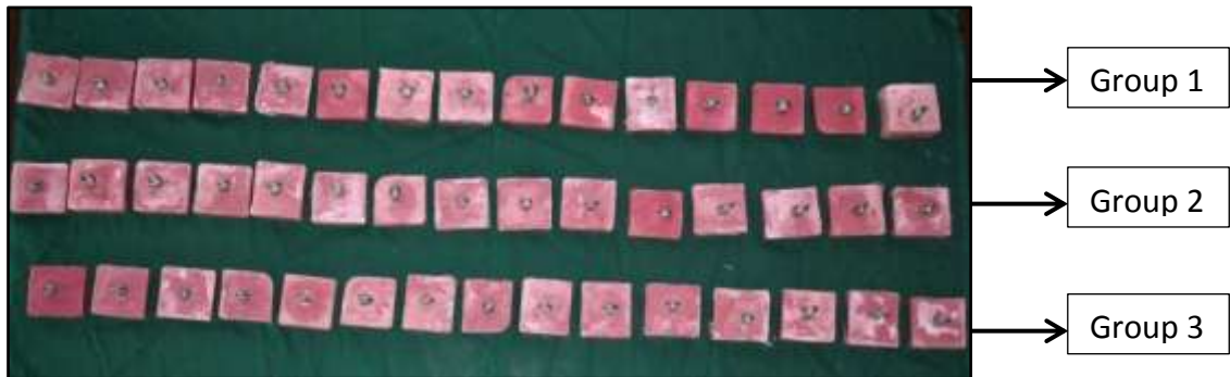
Fig.11 Total 45 DMLS metal crowns cemented on metal dies
