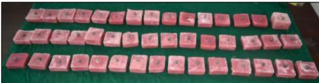
Fig. 5: 45 metal dies submerged in acrylic block
