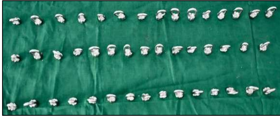
Fig. 7. Final prepared DMLS crowns with loop
