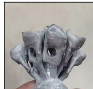
Fig.32.Finally casted Co-Cr copings with loop
