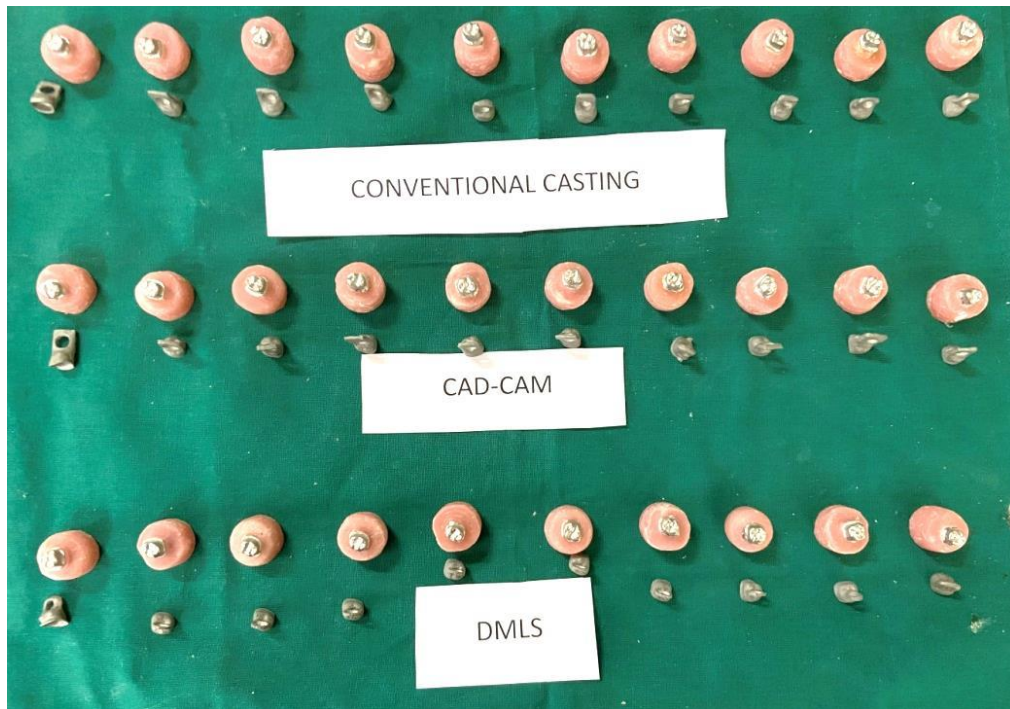
Fig. 39: Finally prepared all three groups METAL crowns with METALLIC loop
