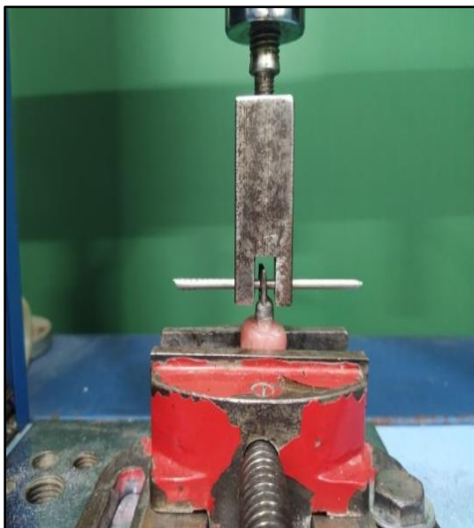
Fig. 43: Retention testing of samples on universal testing machine
