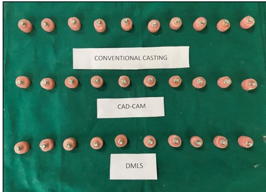
Fig. 30: 30 Metal dies submerged in acrylic block
