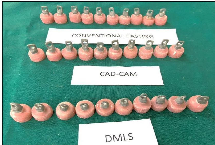
Fig. 42: Total 30 Co-Cr metal crowns cemented on metal dies
