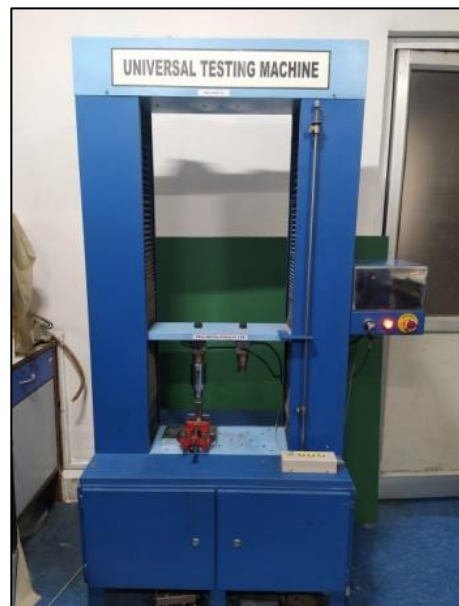
Fig. 43: Retention testing of samples on universal testing machine
