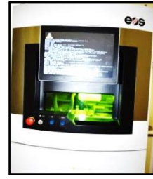
Fig. 38: Sintering of Co-Cr coping in process
