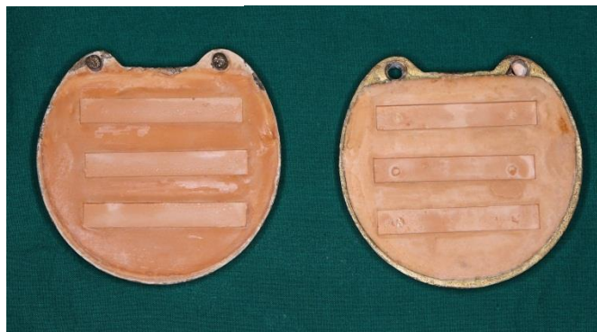
Fig. 23 Preparation of Gypsum mold
