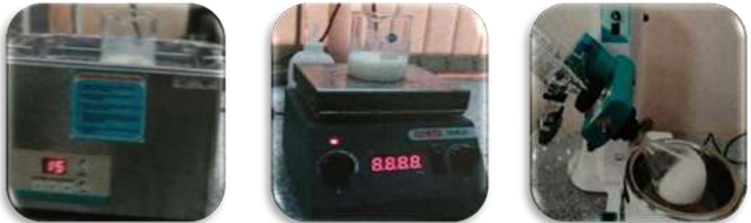
Fig 22: Silanization process of aluminium oxide nanoparticles
