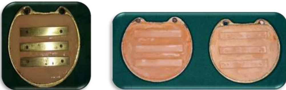
Fig 23: Preparation of gypsum mould to obtain samples
