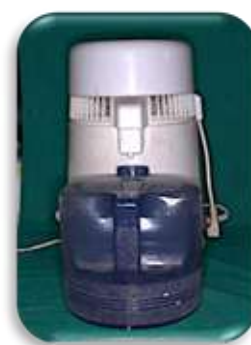
Fig 20: Distilled water plant
