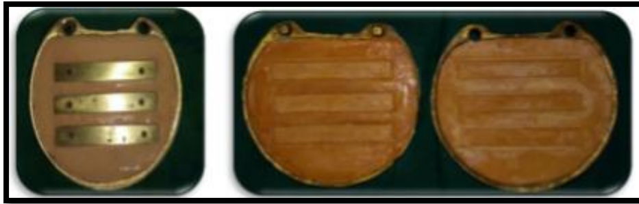
Fig 20: Preparation of gypsum mould to obtain specimens
