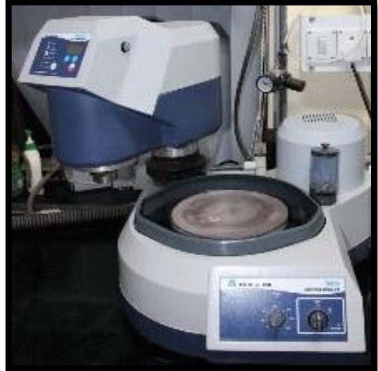
Polishing of samples (Buhler, Germany)
