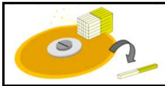
Figure: Cutting of the specimen along X and Y axis and the resulting stick
