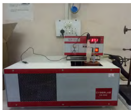
Fig.32. EC cell set-up attached to the wires of potentiostat in chiller (Thermostat) maintained at 37\pm 1^\circ\text{C}
