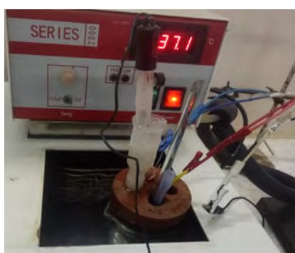
Fig.32. EC cell set-up attached to the wires of potentiostat in chiller (Thermostat) maintained at 37\pm 1^\circ\text{C}
