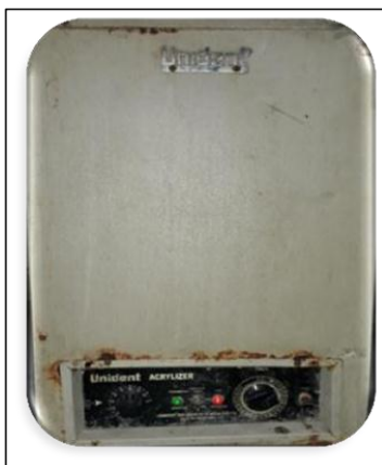
Fig 11: Acrylizer with thermostat
