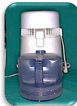
Fig 22: Distilled water plant
