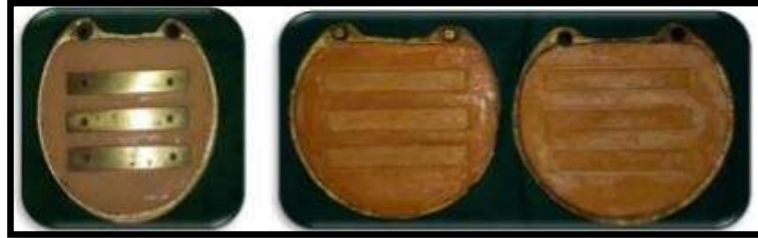
Fig 21: Preparation of gypsum mold to obtain specimens
