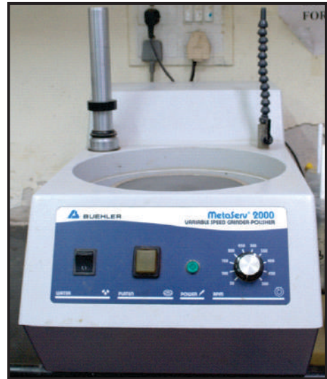
Polishing of samples on Grinder & Polisher (Buehler, Germany)
