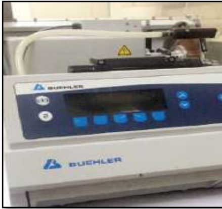
Sectioning of Samples with Isomet Precision Saw (Beuhler)
