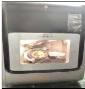
Fig. 8:- Plank of PEEK placed in machine for milling
