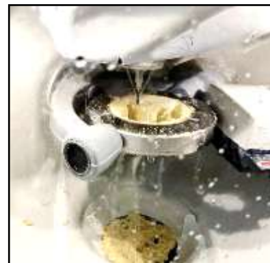
Fig. 9:- Milling by using bur and water spray for coolant
