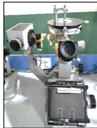
Fig. 4:- Universal Micro Hardness testing Machine
