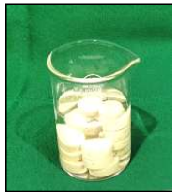
Fig.14:- Samples kept in glass beaker for microwave disinfection
