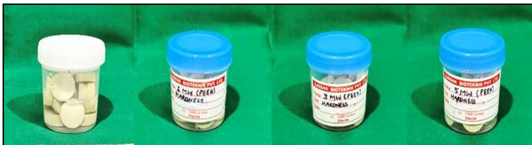
Fig.17:- Samples kept in bottle filled with distilled in which white color denotes without microwave disinfection and colored box labelled for number of microwave disinfection cycle
