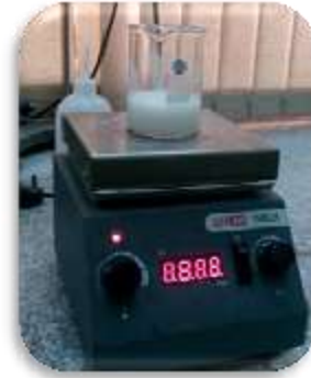
Fig.18 Homogenous dispersion of zirconium oxide nanopowder in monomer
