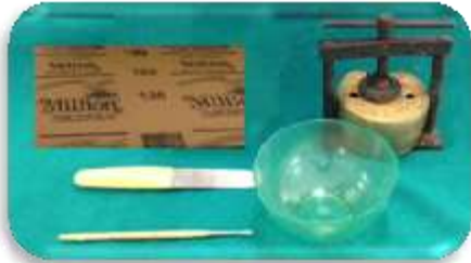
Fig.11 Sandpaper (No.120), rubber bowl, plaster spatula, camel hair brush, varsity flask and clamp
