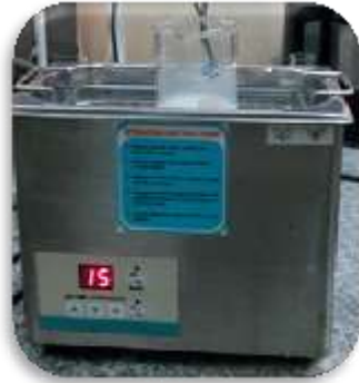
Fig.18 Homogenous dispersion of zirconium oxide nanopowder in monomer
